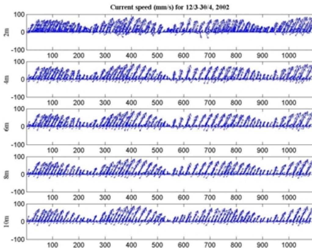
Figure 22. Acoustic Doppler current profiler results for 12/3/02 - 30/4/02.
