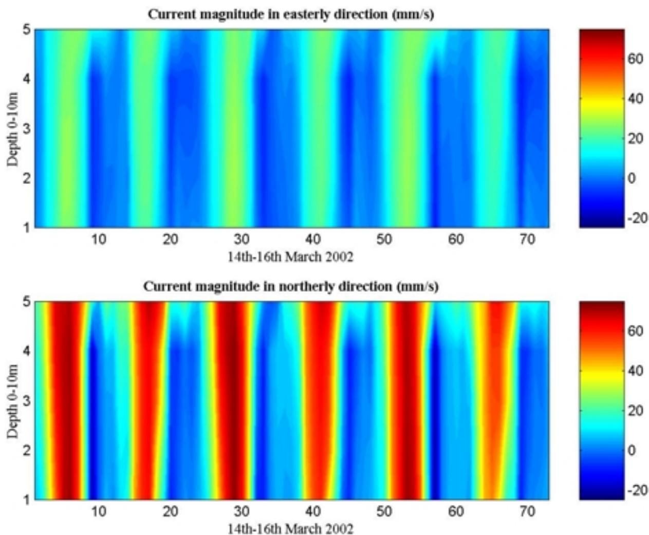
Figure 23. Acoustic Doppler current profile for 14<sup>th</sup>-16<sup>th</sup> March 2002.
