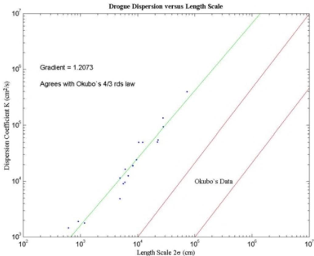
**Figure 11. Dispersion coefficient plotted with length scale and compared to Okubo (1974) data.**
