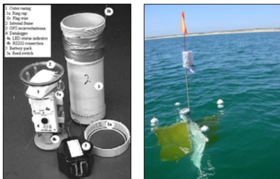
**Figure 3. (a) Drifter components (b) Drogue in water at Point Murat, North West Cape**
